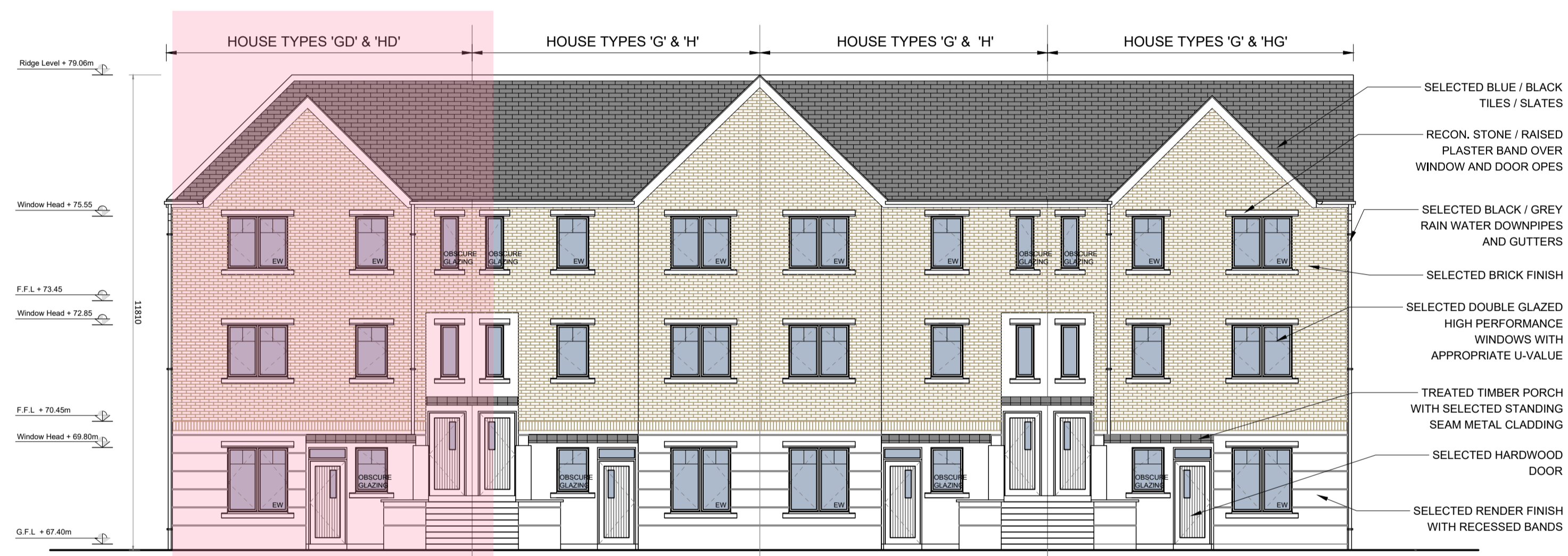
EAST ELEVATION - BLOCK I
